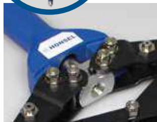
Replaceable nosepieces screwed into the tool.
